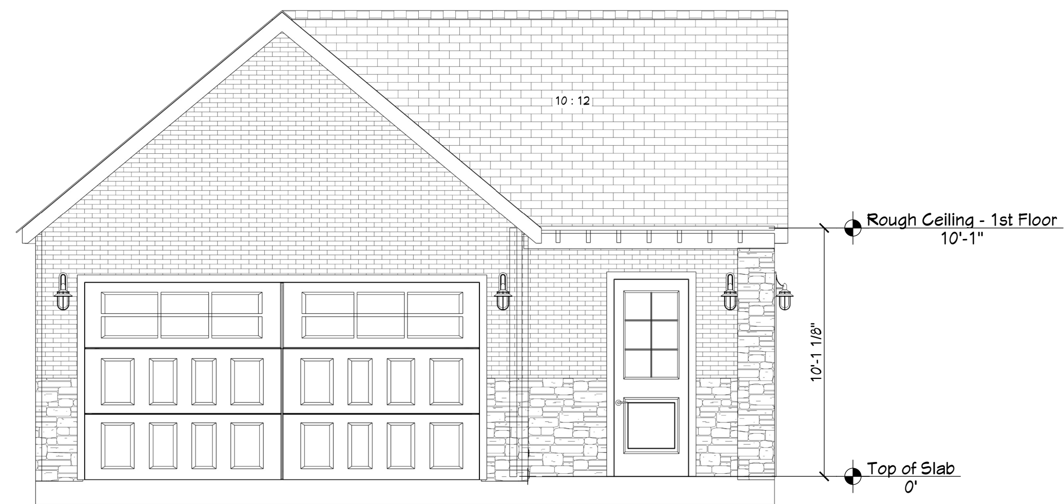
1 DETACHED GARAGE - FRONT ELEVATION SCALE: 1/4"=1'
