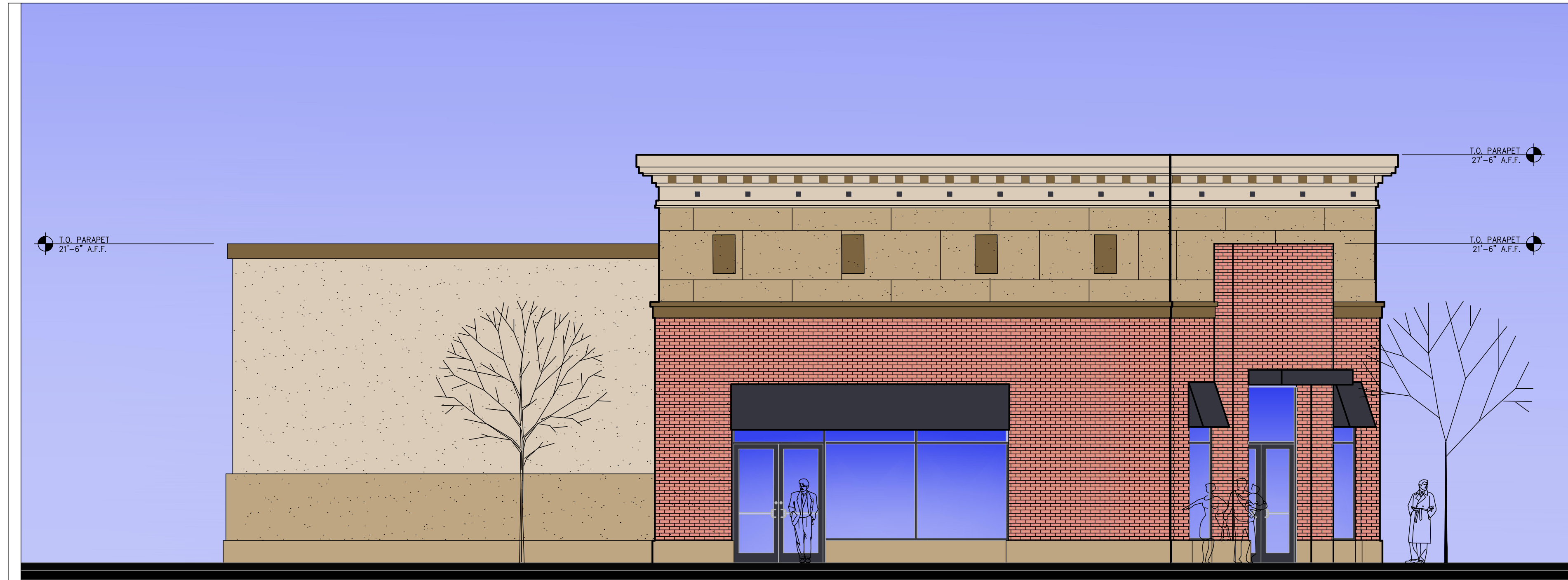
02 RETAIL 2 - WEST ELEVATION SC: 3/16" = 1'-0"
