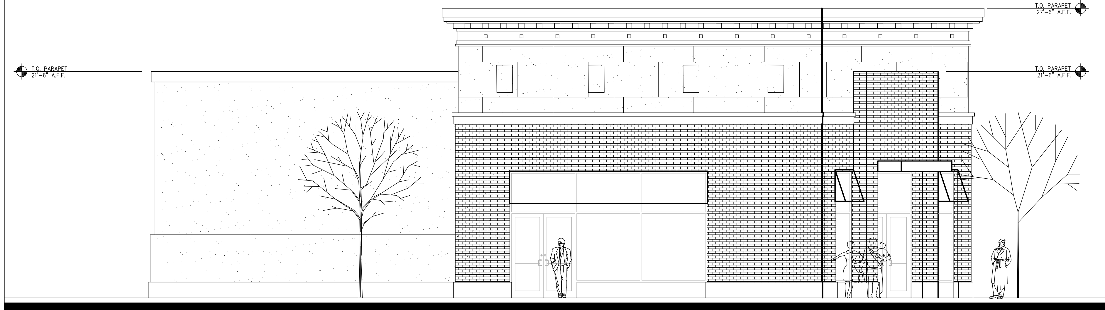
02 RETAIL 2 - WEST ELEVATION SC: 3/16" = 1'-0"
